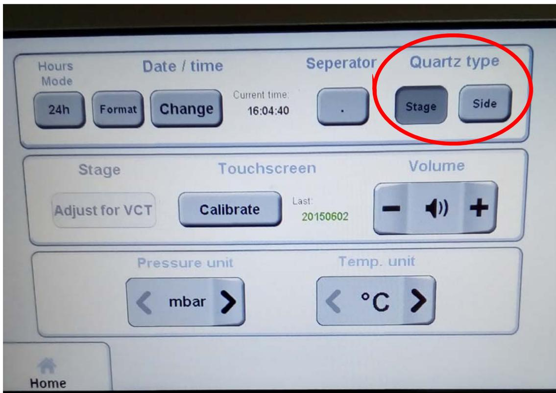
“Stage” means that you set the system for the quartz module physically mounted at the center of the stage.
